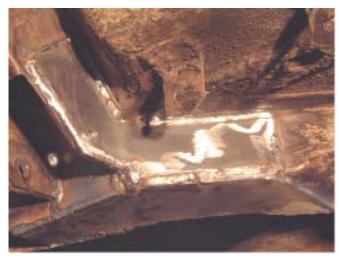
Figure 13. Here we have the finished application to the kit to the rear spring mount. Some minor weld dressing has been done and more can be done, but this gives you the general idea.
