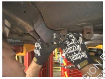
Figure 9. "Fitting" the side piece to the chassis
